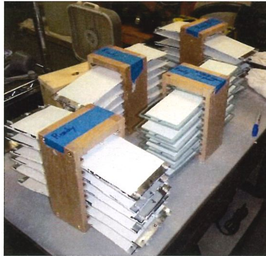
Photo 5: Four sets of specimens in oak rack following coating application before testing
